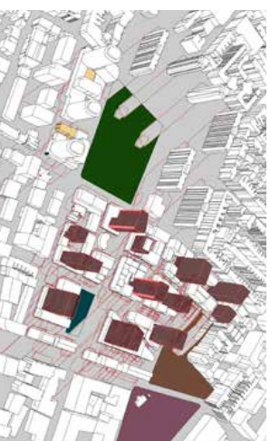
Fig. 7.5.43 Solar access analysis
